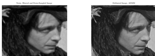
(a) Man (1024x1024) Image; (b) Man (1024x1024) Image; D_s = 3 ; K_S = 5 ; D_s = 3 ; K_S = 5 ; \lambda_{TV} = \lambda_{TV} = 0.2 . Man Blurred/ 0.2. Man Deblurred Image, by Down-Sampled Image. ADMM.
